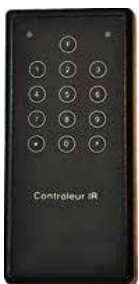
Infrared remote control to configure the automatic system and read the operating data
