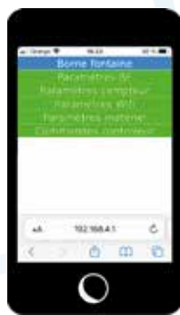
Wireless communication (offline) from any smartphone to configure the automatic standpipe and read the operating data
