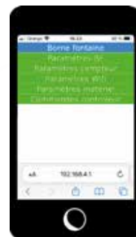
Wireless communication (offline) from any smartphone to configure the automatic system and read the operating data
